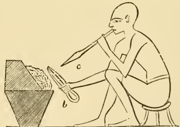
Ancient Egyptian blowing the fire for melting gold, with blow-pipe (c), forceps (b), and firepot having cheeks to confine and reflect the flame.
